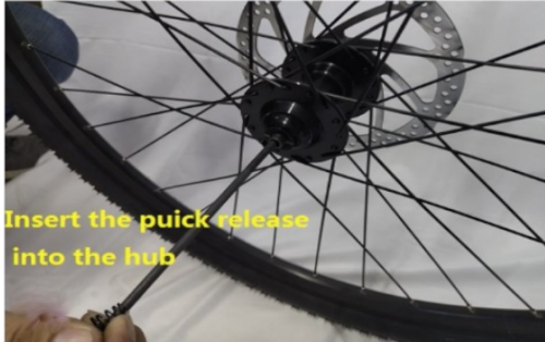
Insert the disc into the gap of the brake and insert the quick release axle into the front hub axle and lock
