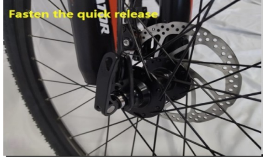
Insert the disc into the gap of the brake and insert the quick release axle into the front hub axle and lock
