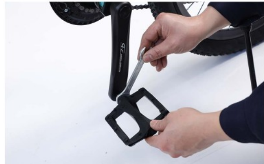
Turn spanner anti-clockwise to fix left pedal
